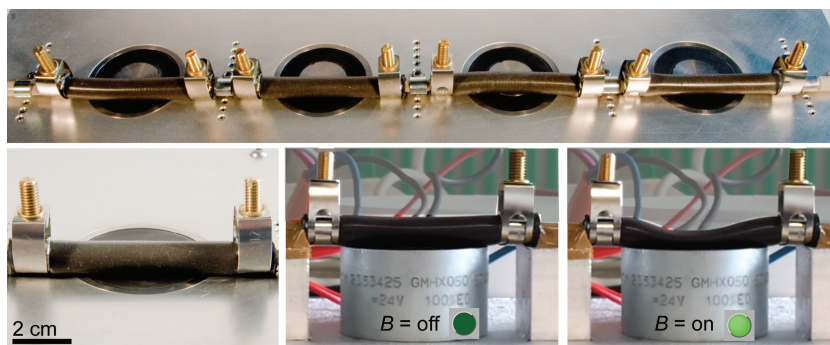
Figure 3. Final apparatus of a magnetic peristaltic pump. Four magnetic tubes were connected to each other and placed on top of 4 solenoids. Tubes were positioned at the edge of the field generating pillar because of the high magnetic field at this position (0.43 T). Turning the electromagnets on, the tube showed a clear contraction towards the magnet and allowed pulsatile movement.
